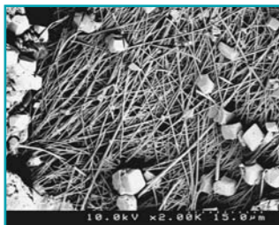
Xypex treated Concrete
