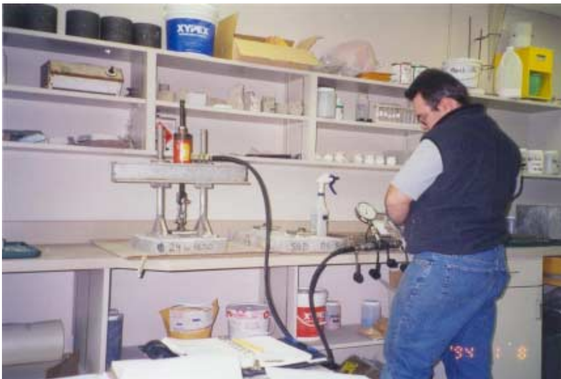
Photograph 1: Bond Pull-off test apparatus and example of prepared concrete slabs.
