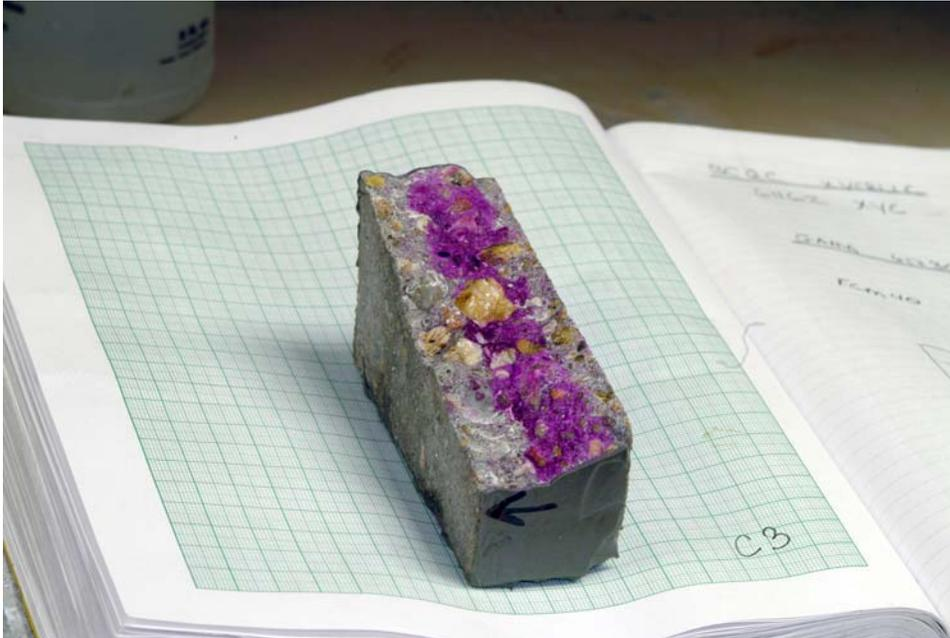
Figure 4: Example of Carbonated Sample
