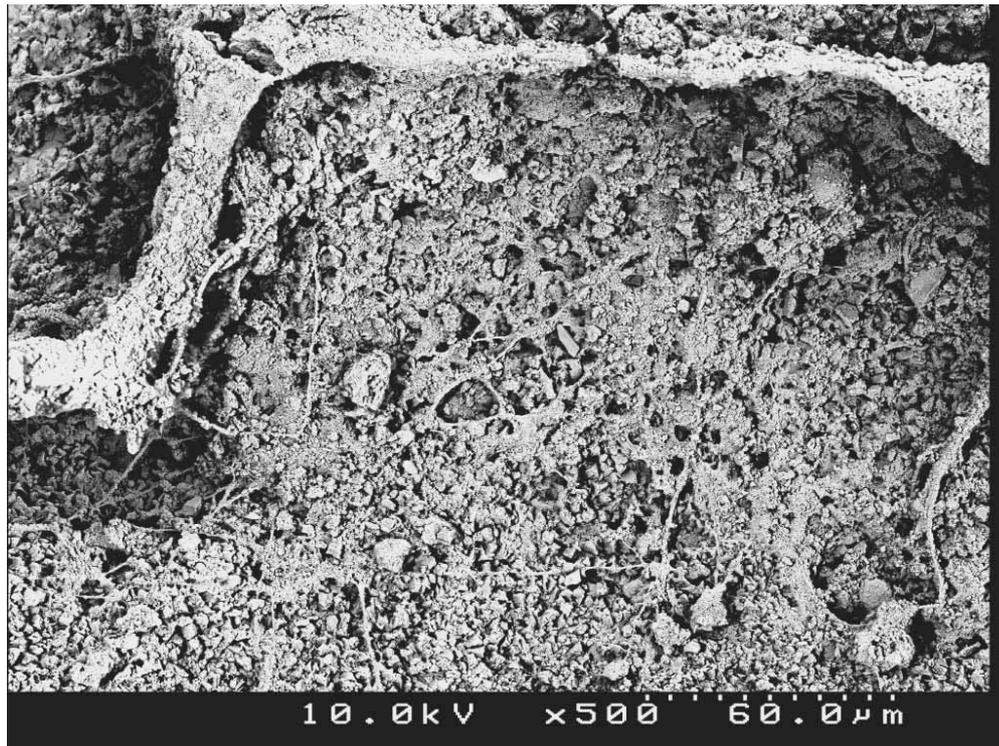
**Fig 7. A Typical Crystalline Product Site on Type-3 Mortar Sample (at X500)**
