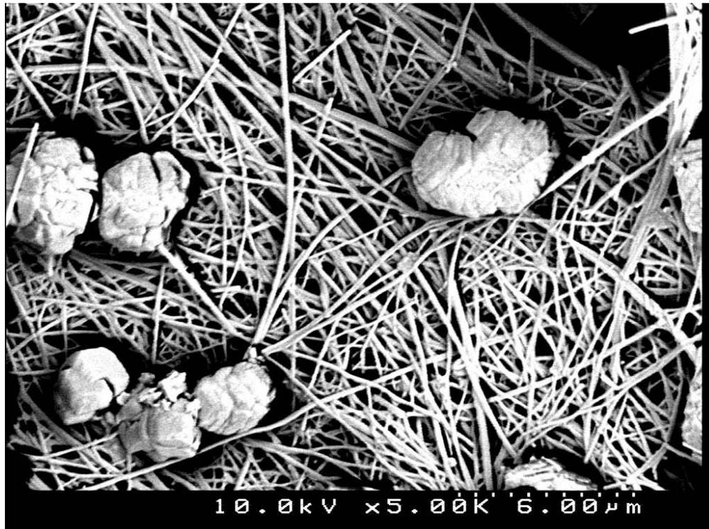
**Fig 3. Crystalline Products in Type-1 Concrete at X 5000 Magnification**
