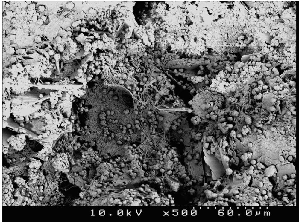
**Fig 1. A Typical Crystalline Product Site on Type-1 Concrete Sample (at X500)**
