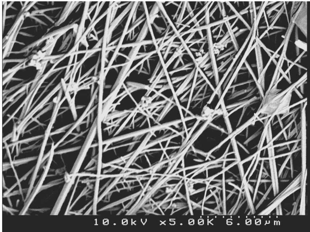
**Fig 6. Crystalline Products in Type-2 Concrete at X 5000 Magnification**
