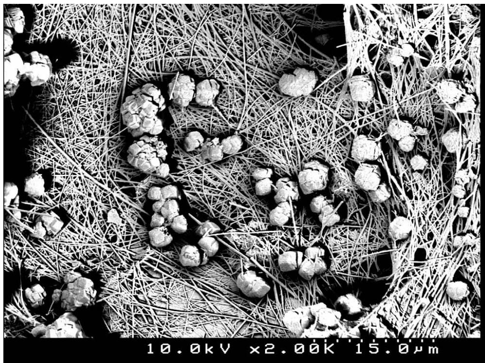
**Fig 2. Crystalline Products in Type-1 Concrete at X 2000 Magnification**
