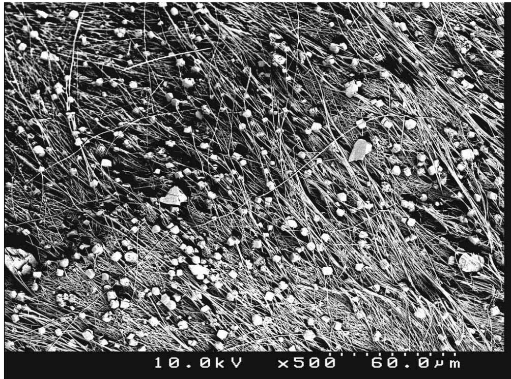
**Fig 4. A Typical Crystalline Product Site on Type-2 Concrete Sample (at X500)**
