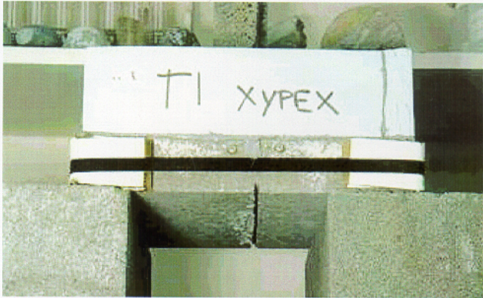
Photograph 2: Xypex Series 1 sample after 100 days.
