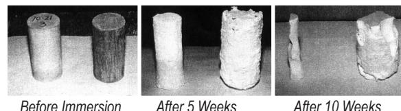
Xypex-treated mortar and untreated mortar were measured for acid resistance after exposure to a 5% H<sub>2</sub>SO<sub>4</sub> solution for 100 days. Xypex suppressed concrete erosion to 1/8 of the reference samples.
