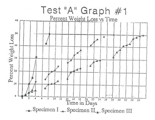
As shown on **Test "A"** Graph #1, the weigh periods along with correspondent weight loss produce a generally linear deterioration of the control sample, as do the weigh periods and weight loss recorded for the admix samples.
