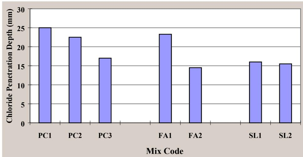
Fig. 8 Chloride Penetration Depths by Nordtest after 35 Days Immersion
