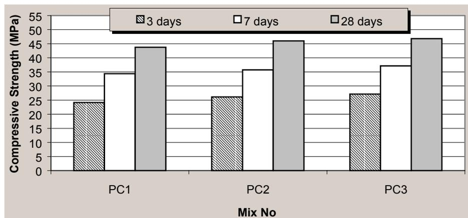
Fig 1. Compressive Strength of Type-GP concretes
