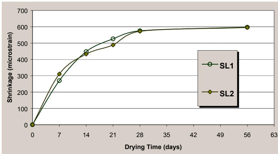
**Fig 5. Drying Shrinkages of Slag Cement Concretes**
