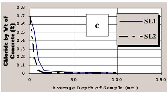
Fig.9 a), b) and c) Chloride Penetration Profiles by Nordtest
