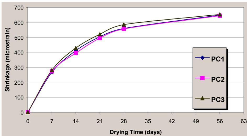
**Fig 3. Drying Shrinkages of Type-GP Concretes**
