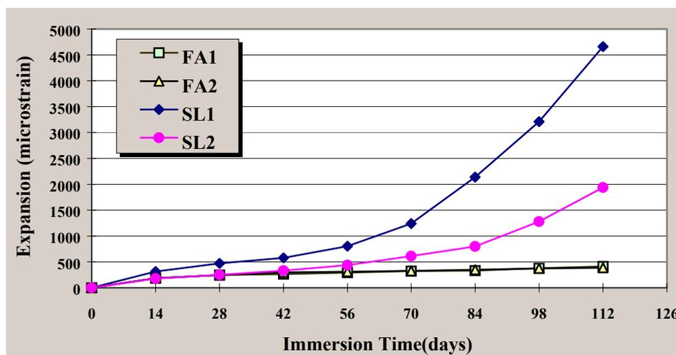
Fig. 7 Length Changes in Sulphate Solution for Fly Ash and Slag Concretes
