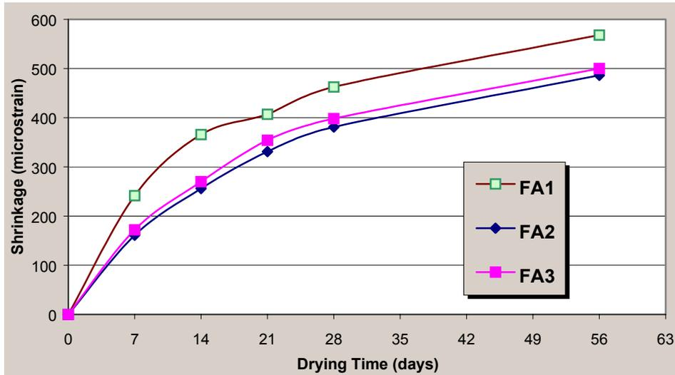
**Fig 4. Drying Shrinkages of Fly Ash Concretes**
