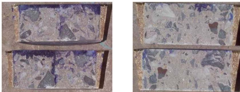
**Fig.10 Water Penetration Depths in Water Permeability Test Specimens Mix-FA1 (left) & Mix-FA2 (right)**
