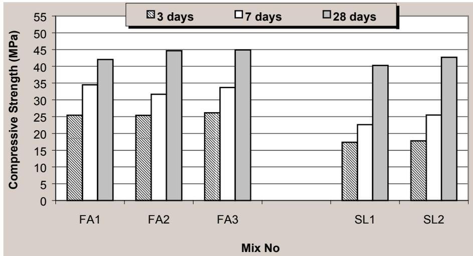
**Fig 2. Compressive Strength of Fly Ash Concretes and Slag Concretes**
