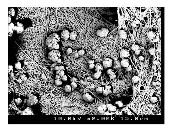
Fig 2. Crystalline Products in Type-1 Concrete at X 2000 Magnification
