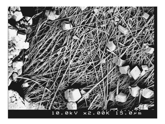
Fig 5. Crystalline Products in Type-2 Concrete at X 2000 Magnification
