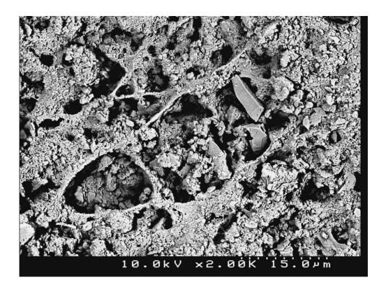
Fig 8. Crystalline Products in Type-3 Mortar at X 2000 Magnification
