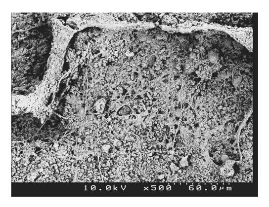
Fig 7. A Typical Crystalline Product Site on Type-3 Mortar Sample (at X500)
