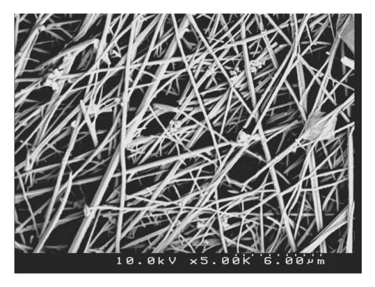
Fig 6. Crystalline Products in Type-2 Concrete at X 5000 Magnification
