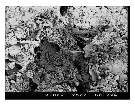
Fig 1. A Typical Crystalline Product Site on Type-1 Concrete Sample (at X500)
