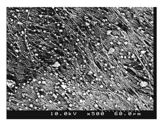
Fig 4. A Typical Crystalline Product Site on Type-2 Concrete Sample (at X500)
