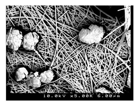
Fig 3. Crystalline Products in Type-1 Concrete at X 5000 Magnification
