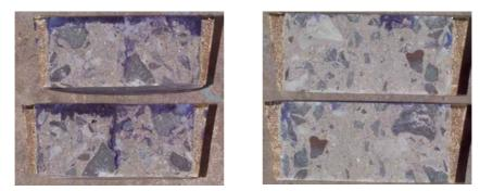
Fig 3.2-1 Water Penetration Depths in Water Permeability Tests Mix-FAC (left) & Mix-FAX1 (right)
