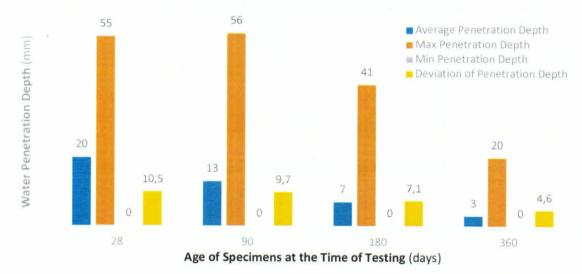
The analysis of the results shows that the average water penetration depth into the hardened concrete at the nominal strength dates of 28 and 90 days, is at 20 mm and 13 mm respectively. This confirms the relatively good water tightness of the tested concrete.
